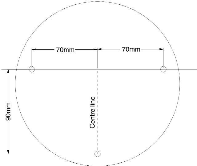
On the upper line, drill holes 70mm (2¾") from the centre line, using a 6 mm (¼") masonry bit, and insert a wall plug.
