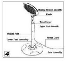
Attach the heating element assembly to the top of the pole. Clamp tightly using the fixing knob.
