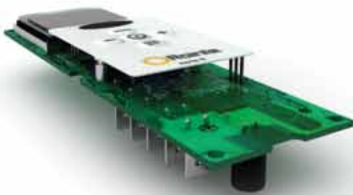
K Series control panel: the brain that controls our radiators.
